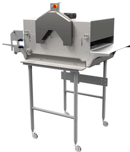
The outfeed side, where washed trays are collected.
