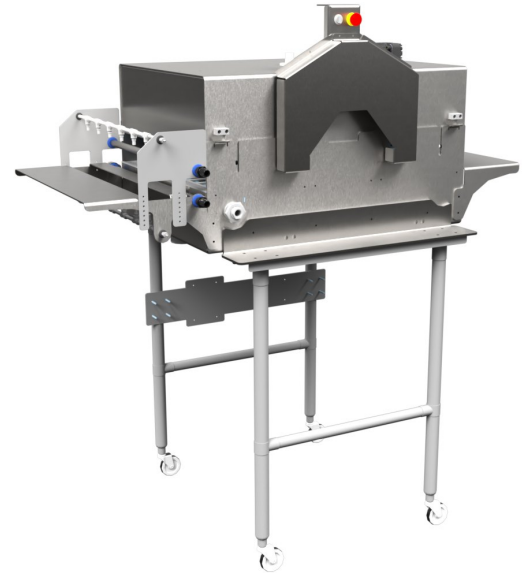
The intake side, where trays are loaded.
